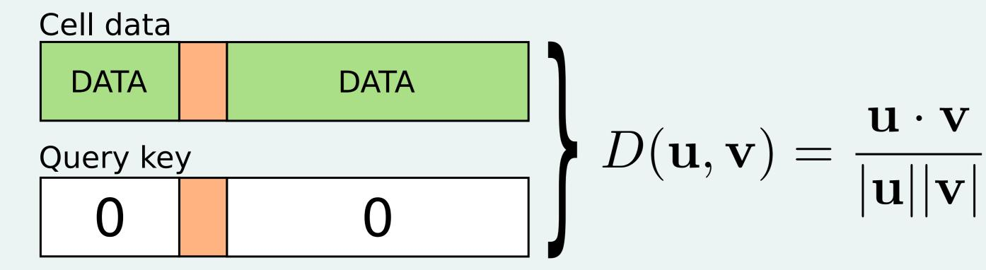
Solution: explicit masking of both the data and the query key
